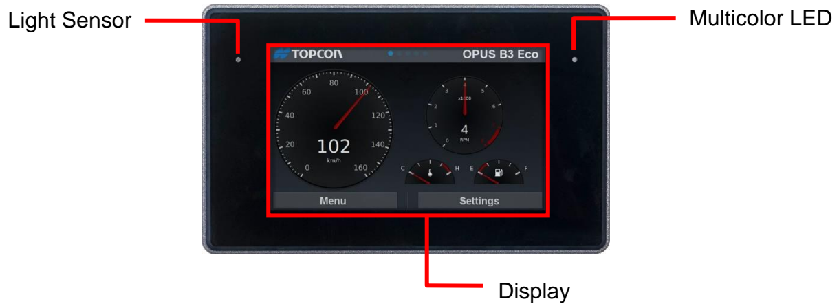
Fig. 3.1: Schematic diagram of the OPUS B3
