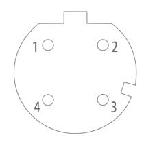
Recommended mating connector type according to IEC 61076-2-10: MM 004-G**x**1-B x) A, C, I, P, R or S-type
