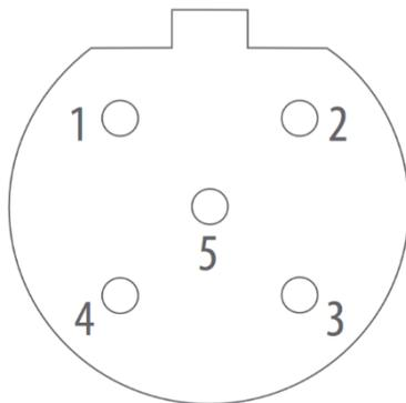
Ethernet connector, M12, female, 4 pins, d-coded,
